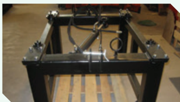
The optional CM1600M side shifter increases the reach by 55 cm and speeds up evasive manoeuvres.
